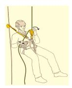
Ensure that the ropes and other components are properly arranged/protected to avoid abrasion and are not in contact with chemicals, hot surfaces, sharp objects or exposed to wet environment and direct heat of sunlight.
